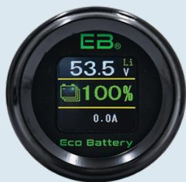
**CALIBRATION:** The SOC meter does not require calibration by the end user, as it receives its data directly from the battery's BMS. The BMS will perform a self-calibration at the end of each full charge cycle and periodically during rest periods. Accuracy is +/- 5%.
